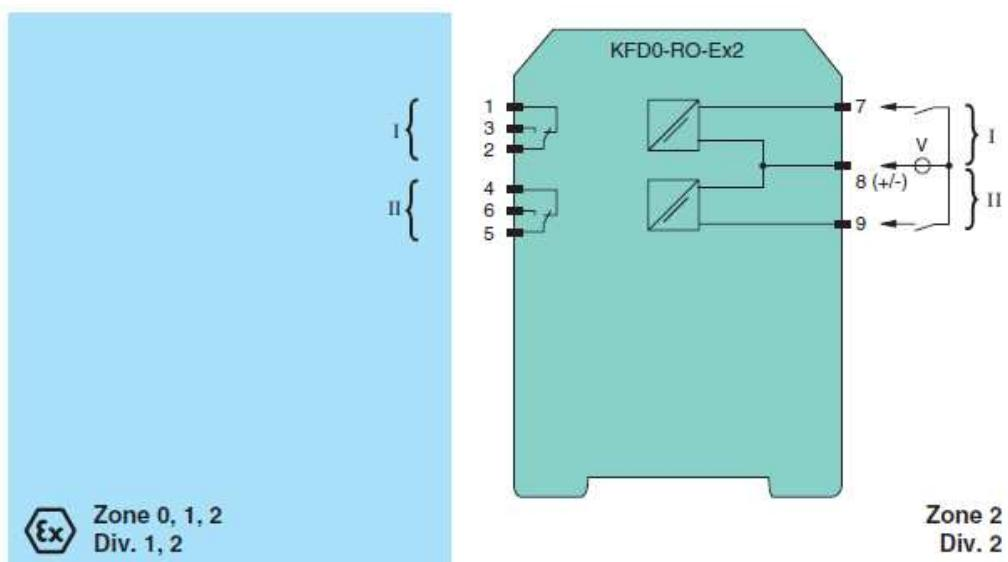
Fig. 1: Connection of the KFD0-RO-(Ex)2
