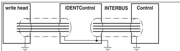
The cable shielding is used to discharge electromagnetic interference. When shielding a cable, you must connect both sides of the shield to ground with low resistance and low inductance.
