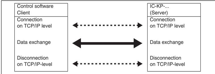
A connection must be established on the TCP/IP level before data can be exchanged. From this point onwards, commands can be sent from the client to the IC-KP-B12-V45 device.
