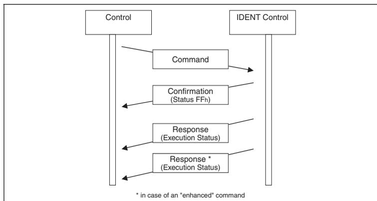
To execute a command, the control software (client) sends a command to the identification system. The server then sends confirmation of receipt (TCP/IP and Ethernet/IP only). The server sends the response after the command is processed.
