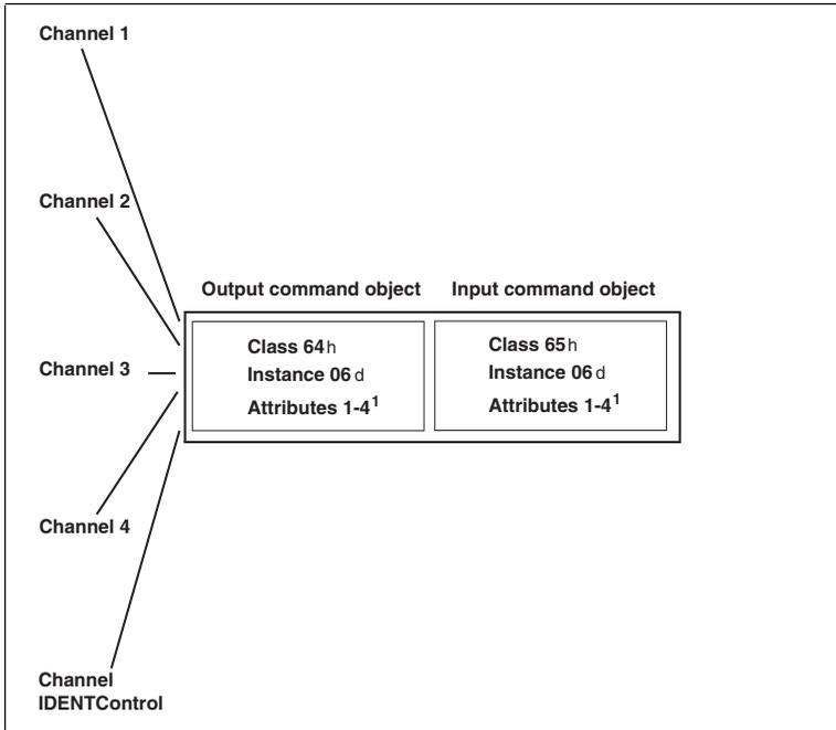
The five IDENT channels (four R/W heads, one configuration channel) are addressed using an input and an output instance, with the advantage that the controller requires less memory.
