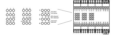
There are 3 indicator fields on the faceplate, each with 12 LEDs. The **right** field shows the status of the 4 read/write heads (IVH 1 ... 4); each head is assigned 3 LEDs. The green LEDs indicate whether the corresponding head is on (IVH active). A yellow LED indicates when a program, write or read sequence has been successfully completed (IDC detected). The red LEDs (reserve function) are for future functions.
