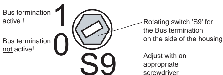
Fig. 5.4: Rotary switch S9 for the termination of the bus.
