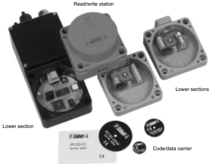
Figure 4.2: Overview of the structure of the inductive identification system IDENT-I System P.
