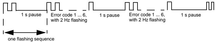
Only the LEDs of the channel that has an error will flash.
