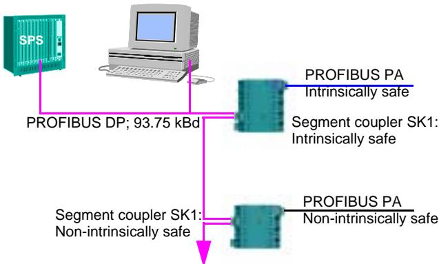
If the SK1 segment coupler is used, the transfer rate for the PROFIBUS DP is fixed at 93.75 kBd. In this case, if type A cable is used for the PROFIBUS DP the PROFIBUS DP segment can be up to a length of 1200 m. The length of the PROFIBUS PA segment depends on:
