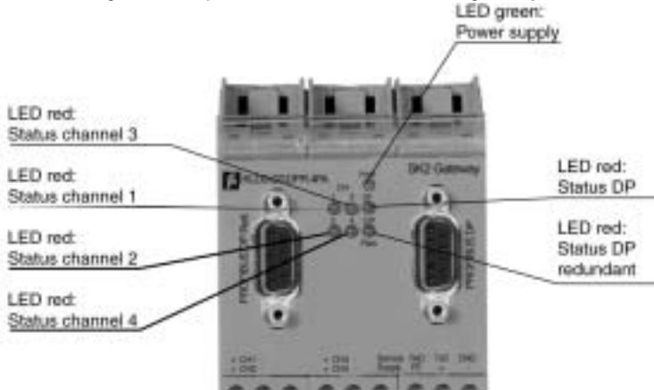
In normal operation, the LEDs should display the following state if there are no errors:
