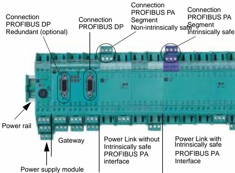
The gateway is used to convert the PROFIBUS DP protocol to the PROFIBUS PA protocol and back.
