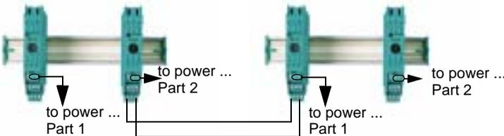
Power Links that are assigned to PROFIBUS PA channels 2 through 4 must not be located on the same Power Rail segment as Power Links of the PROFIBUS PA channel 1. This automatically separates power supply segments from each other and provides separate power feed modules for these PROFIBUS PA channels to use.
