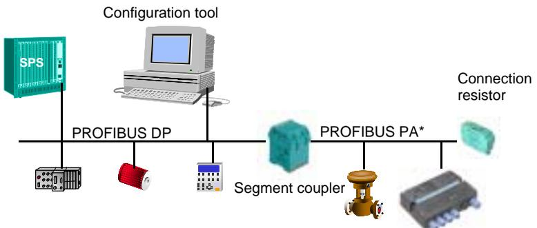
\*depending on the used segment coupler type the PROFIBUS PA segment can be intrinsically safe.
