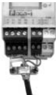
Figure 5.1: Shielding the data cable to the read/write heads
