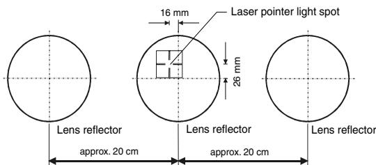
Figure 5.9 Recommended arrangement for horizontal beam adjustment because of uneven motion
