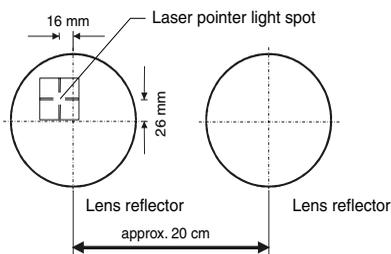
Figure 5.8 Minimal arrangement for distances from 120 m to 240 m (2x lens reflector R 140)
