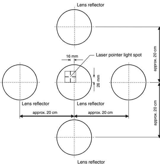
Figure 5.10 Recommended arrangement for horizontal and vertical beam adjustment because of rough surface and uneven motion
