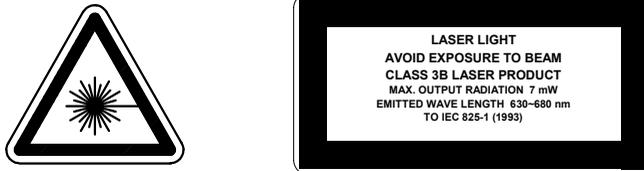
Figure 3.2 Laser diode class label
