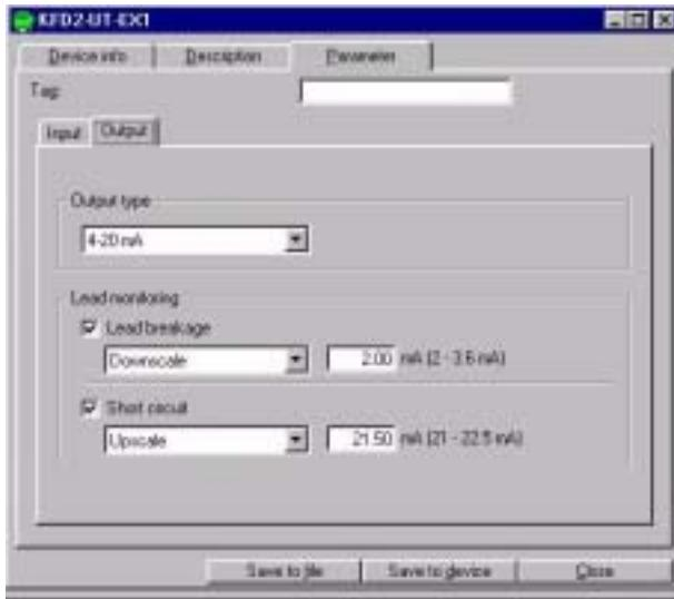
Here too, once configured in the dialog, the new parameters can be saved to the project file or to the device using the buttons below. The window can be closed using the button on the right or the standard  button, upper right,
