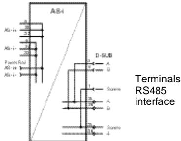
The AS-i master with an RS485 interface transmits and receives across pins 3 and 8 of the SUB-D connector.
