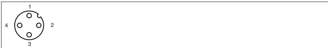
Pin assignment of the M12 socket for RS 232
