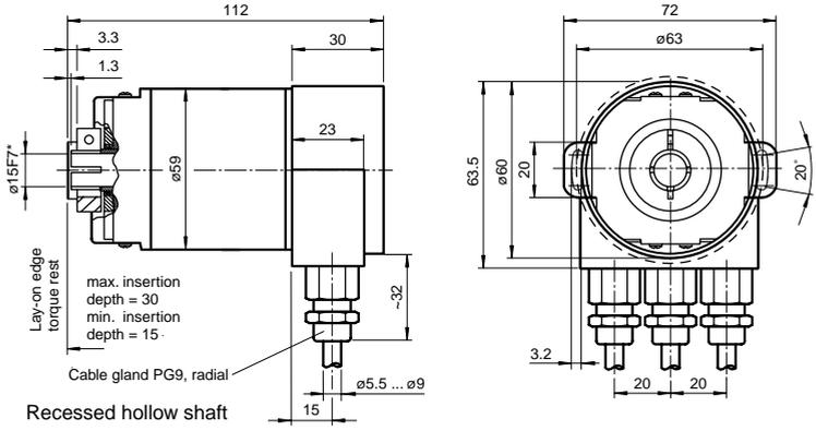
\* shaft can be reduced to  $\varnothing 10F7$  or  $\varnothing 12F7$  by using an adapter
