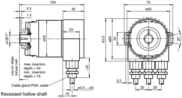
\* shaft can be reduced to  $\varnothing 10F7$  or  $\varnothing 12F7$  by using an adapter
