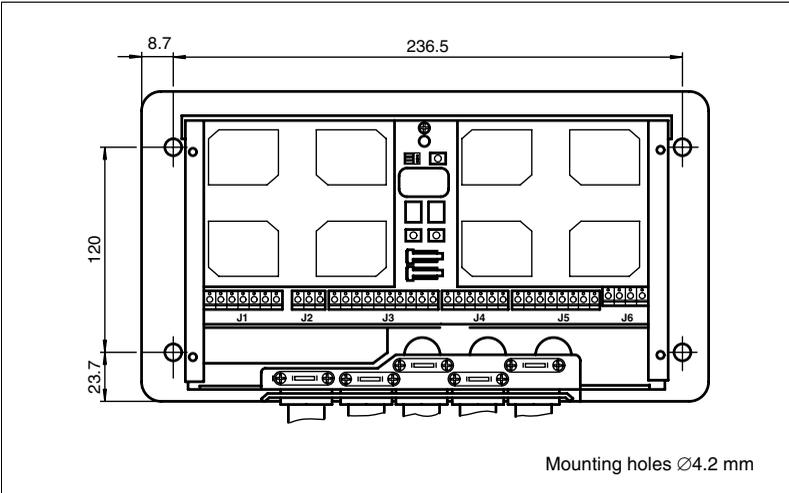
Bild 5.2: MTT-S3 mounting hole locations
