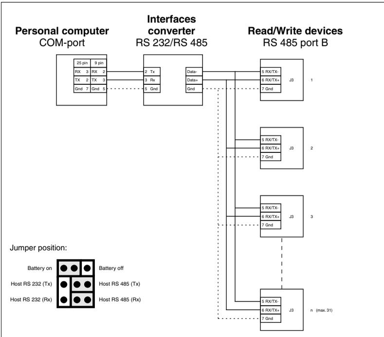
Bild 5.8: Multipoint connection to PC/host via the RS 485 interface
