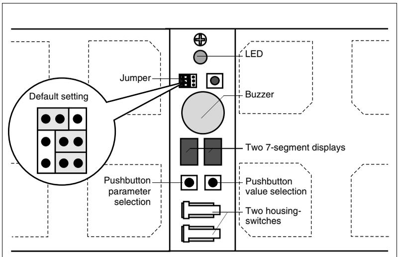
Bild 7.1: Control panel's location
