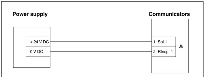
Bild 5.10: Connection of the supply voltage
