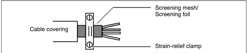
Bild 5.6: Proper grounding using strain-relief clamps
