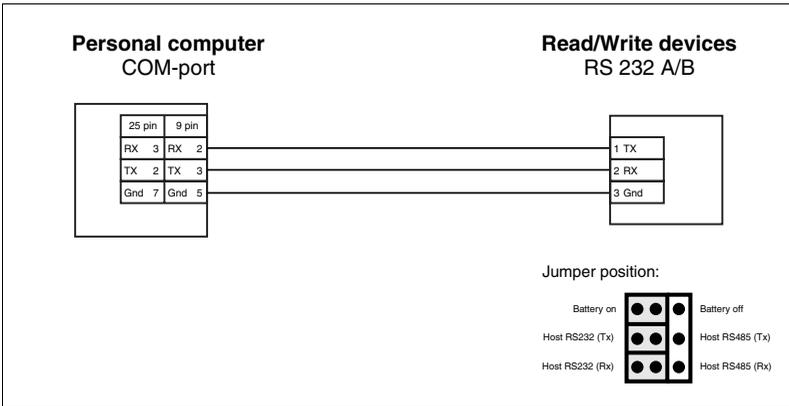
Bild 5.7: Connection to PC/host via one of the RS 232 interfaces
