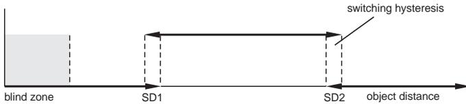
**5.3 Reflex photoelectric barrier mode (R)**
