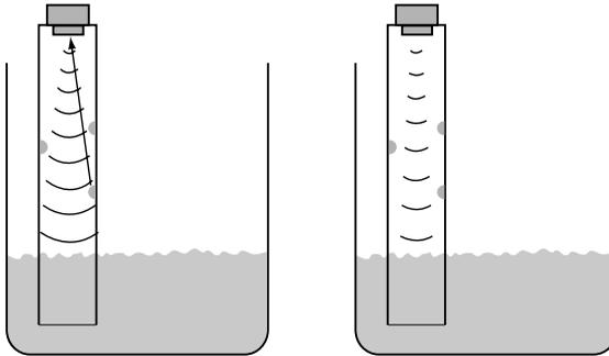
Reflection at disturbance targets    Disturbance target suppressed
