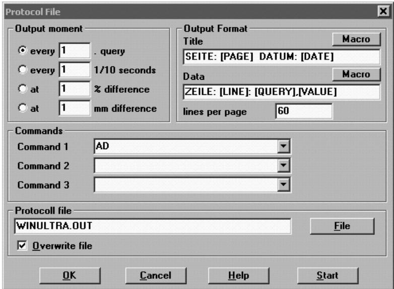
Figure 5.1: Input mask for defining and formatting the log file
