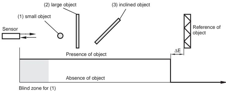
**5.4 Double switching point mode (H) switch output (hysteresis mode)**
