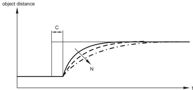
The weighting exhibits typical low-pass response. After a sudden change in the measured values (distances/propagation times), the evaluation results are retrospectively brought into line with the current values on the typical curve. The larger the weighting factor  $N$  chosen, the shallower will the curve be, and in turn the longer the tracking will take.
