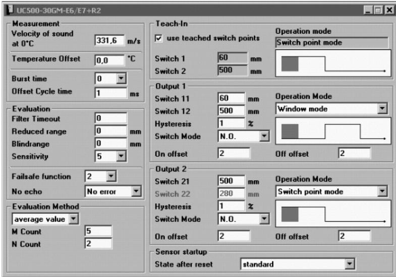
Figure 4.1: Parameter setting window for example UC...-30GM-E6R2/E7R2...
