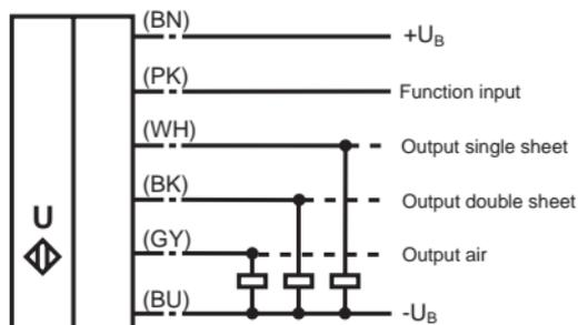
Fig. 7.1: Electrical connection
