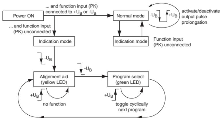
Fig. 6.1: Parameter assignment
