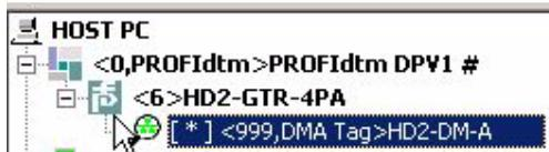
3. To assign a tag to the Advanced Diagnostic Module, open the offline dialog of HD2-GTR-4PA.
