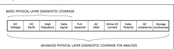
Fig. 3-3: Basic and advanced physical layer diagnostic coverage
