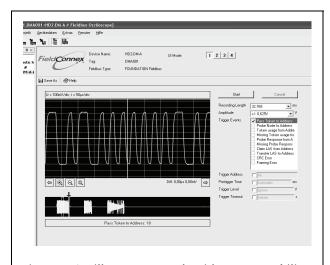
Fig. 4-3: Oscilloscope example with zoom capability, fieldbus specific trigger point options and digital storage.
