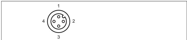
Figure 4.5 External illumination pin assignments
