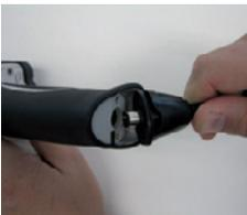
4. Press the 8-pin DIN plug, including spacer disk and protective cap, onto the socket.
