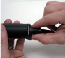
5. Use a screwdriver and the screws provided to fasten the protective cap onto the bottom of the handle.
