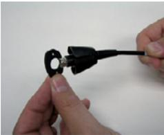
When the spacer disk snaps onto the DIN plug, it is attached correctly.
