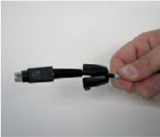
2. Attach the spacer disk to the 8-pin DIN plug.
