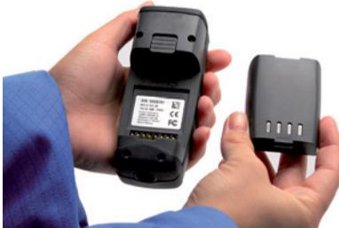
2. Slide the plastic tab on the battery into the corresponding recess on the Handheld.
