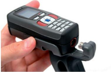
2. Push the Handheld back until the plug on the handle enters the cable connection socket on the Handheld.
