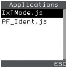
All JavaScript applications saved on the device are displayed in the **Applications** menu. The two programs IxTmode.js and PF\_Ident.js are required to operate the device as a Handheld.
