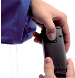
4. Push the battery in the Handheld, hold in position and release the locking device so that the battery engages.
