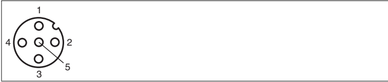
Figure 4.3 Slave connection (M12 socket)
