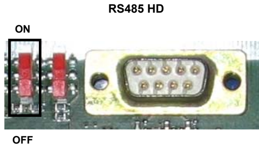
Figure 11 – RS485 HD Termination Resistance Switch
