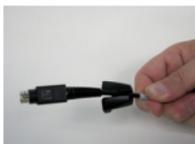
2. Align the 8-pin plug so that it fits into the socket on the handheld.
