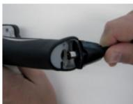
3. Press the 8-pin DIN plug and protective cap onto the socket.
