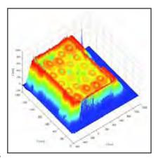
place during the time when the robot is feeding the gripped object to the machining process. During every measurement movement, the shape of the bin is also checked and the data for avoiding collision is integrated into the communication with the robot or the handling unit.
