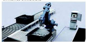
This example describes an application with a leading global automotive group in which untreated brake disks from a bin had to be fed to another machining process. Until a short time ago this activity was carried out by employees who would manually pick the brake disks out of the bin. The task had the following conditions and complexities:
