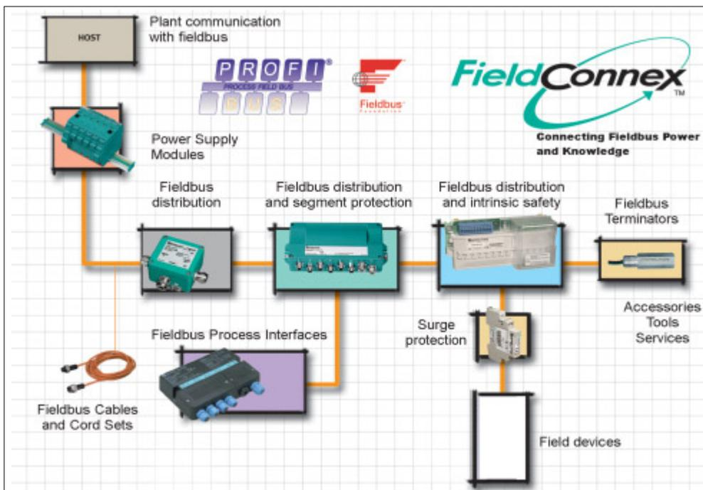
Figure 15: Topology concepts for fieldbus communication based on the example of FieldConnex™.
