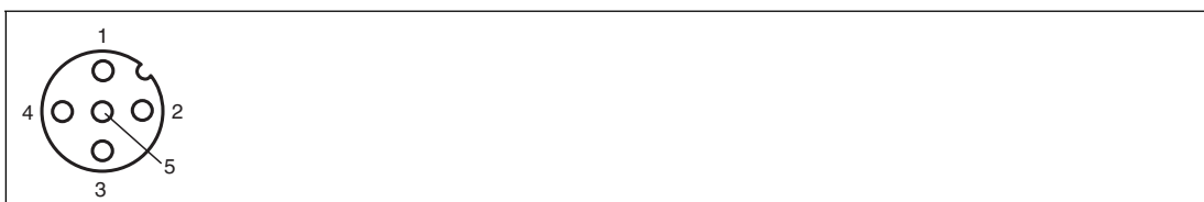
Pin assignment of the M12 socket for RS 485
