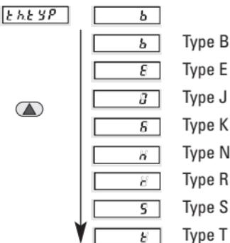
For the thermocouples specified here, scaling slopes with 24 pairs of values are stored in the unit. Intermediate input values between the stored pairs of values are linearly interpolated.
