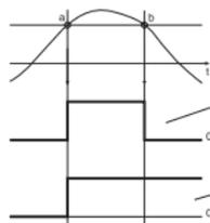
Alarm    a: threshold exceeded
