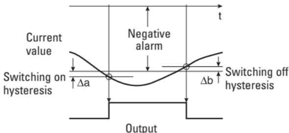
Switching on value = alarm - switching on hysteresis  $\Delta a$
