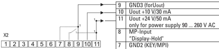
1 Alternatively connect directly to DC supply
