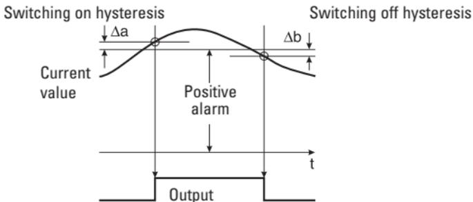
Switching on value = alarm + switching on hysteresis  $\Delta a$
