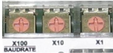
**Figure 3 – Address Selection Switches**
