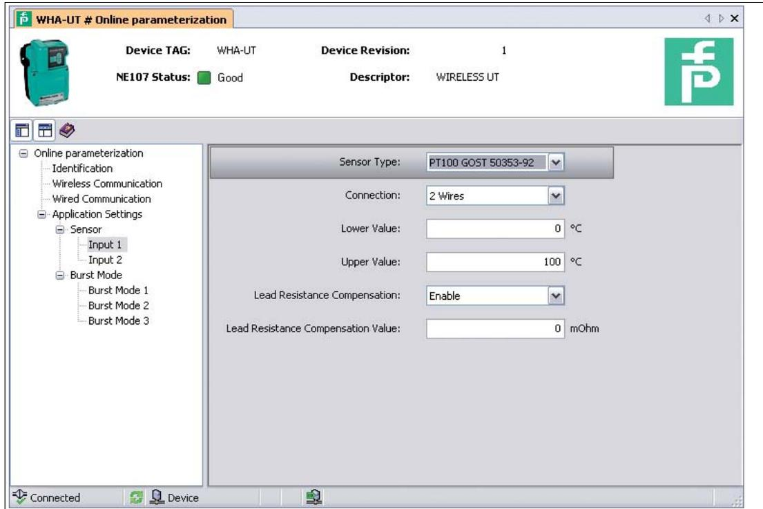
Figure 5.7 Application Settings > Sensor > Input 1 (Selected Sensor Type: RTD)
