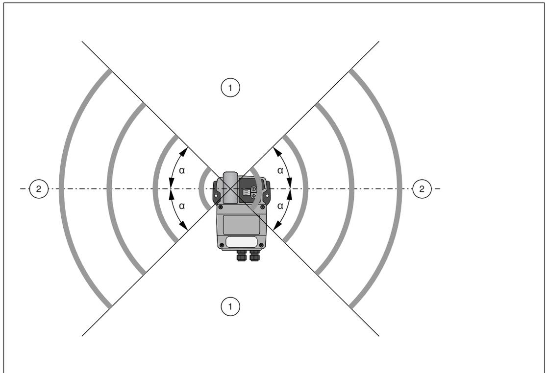
Figure 3.3 Wave propagation, schematic representation (alpha = approx. 45°, may vary considerably)
