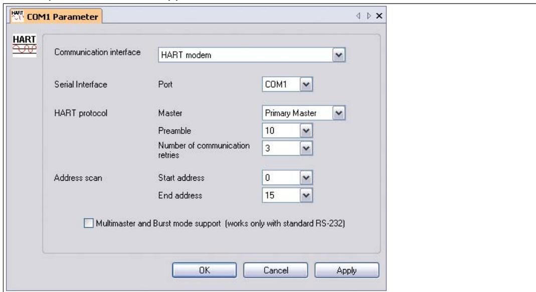
Figure 4.6 Parameter window of HART communication DTM
