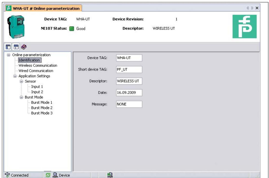
Figure 5.3 Identification parameters
