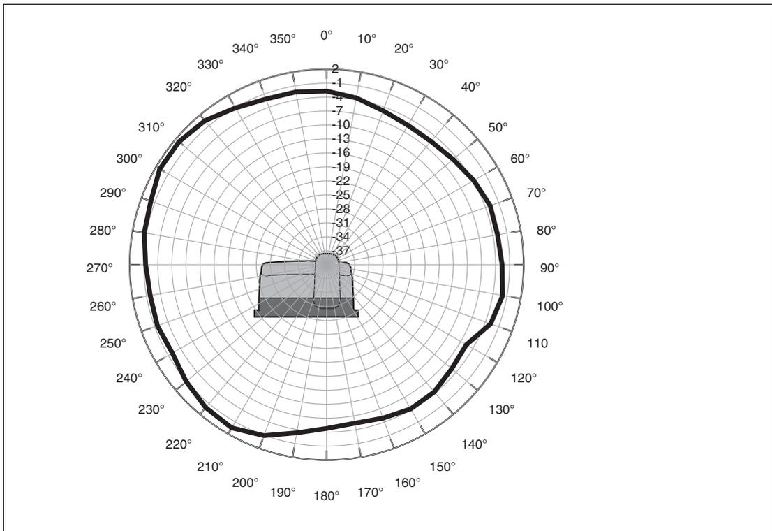
Figure 3.2 Antenna gain (top view, 2450 MHz, dBi)
