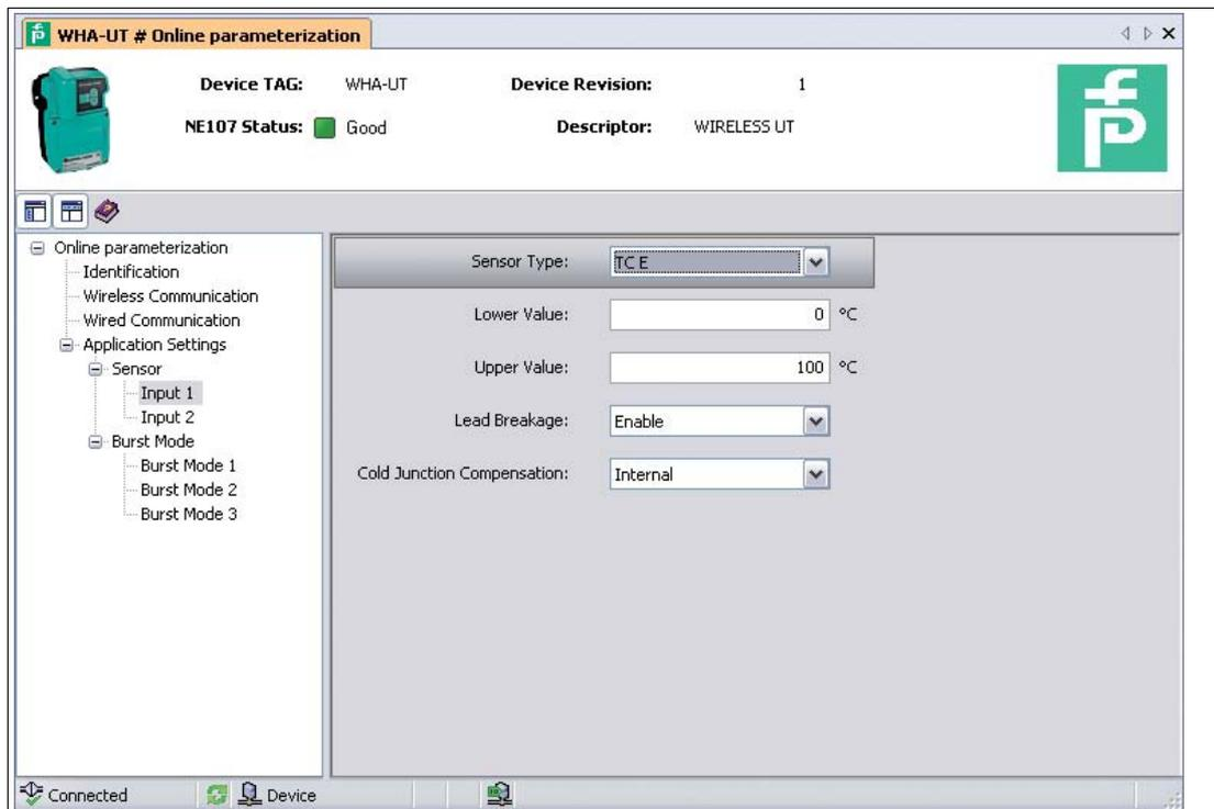
Figure 5.8 Application Settings > Sensor > Input 1 (Selected Sensor Type: TC)
