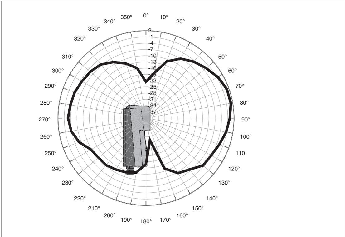
Figure 3.1 Antenna gain (side view, 2450 MHz, dBi)
