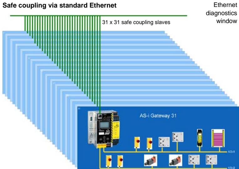
For Safe Link the Gateways are connected over the Ethernet diagnostics interface (10 Mbit/s, half-duplex) and a switch. In the case of PROFINET and EtherNet/IP+Modbus TCP, instead the fieldbus interface can be used for Safe Link.
