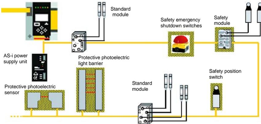
Fig. 4-1. Safe and standard components in an AS-i network
