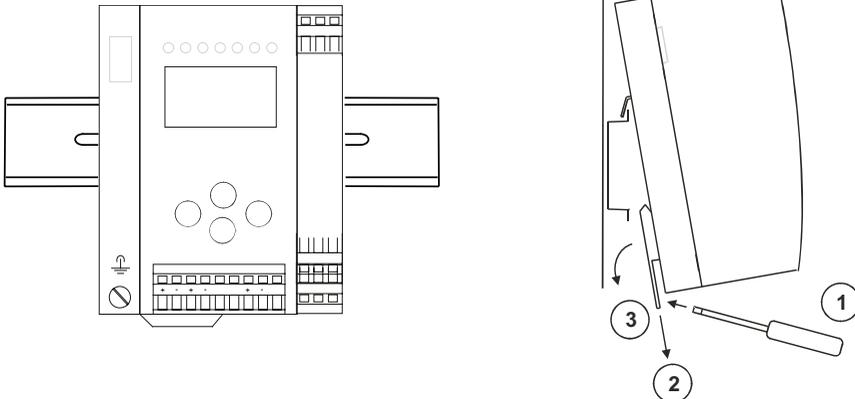
To remove, press the holding clamps [2] down using a screwdriver [1], press the unit firmly against the upper rail guide and lift out.
