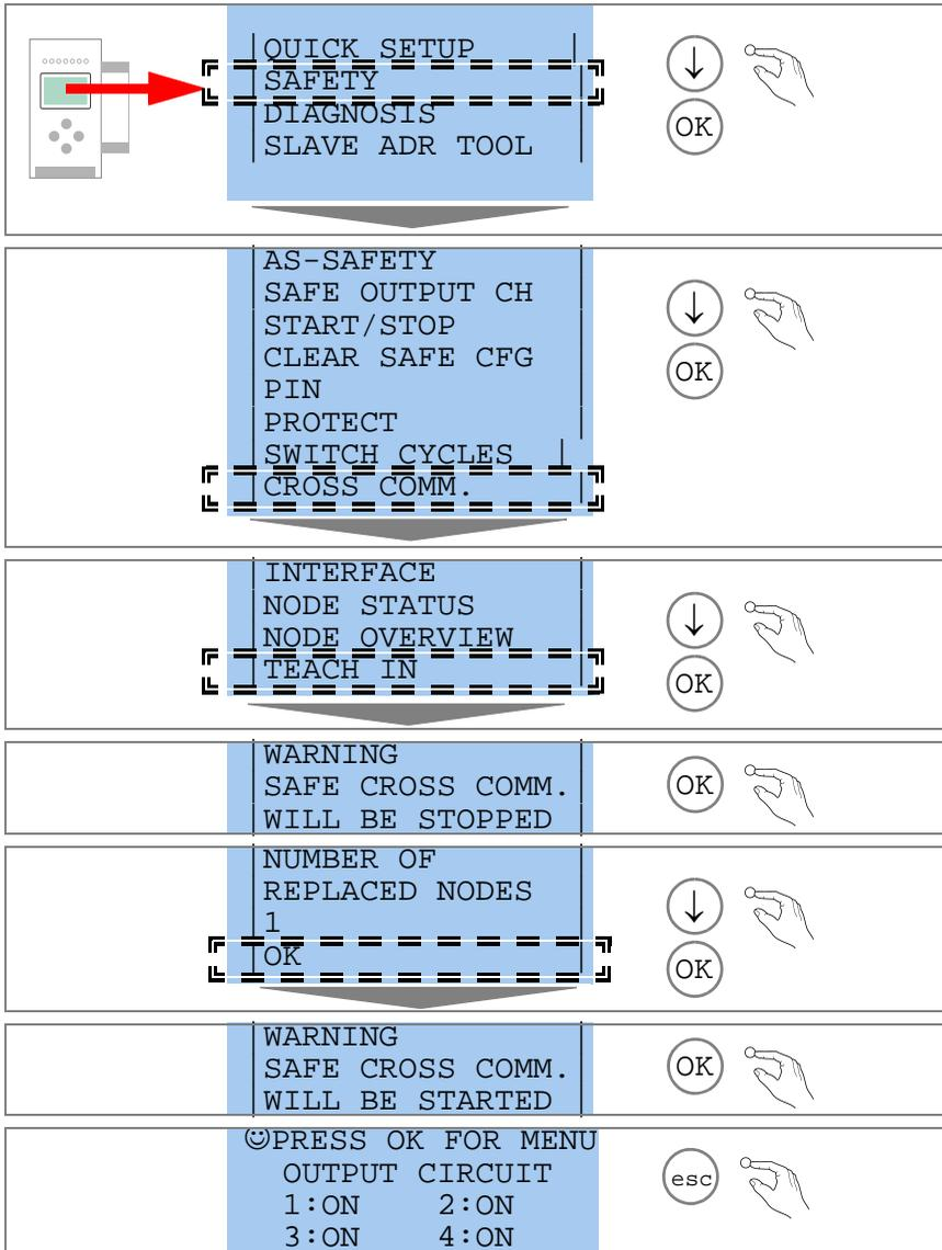
6.12 Replacing the monitor
