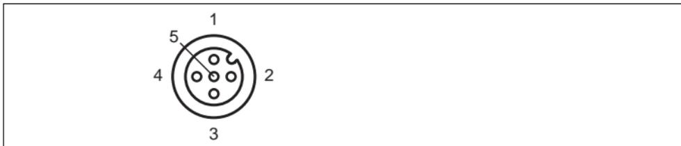
Figure 2.3: Trigger sensor connection layout
