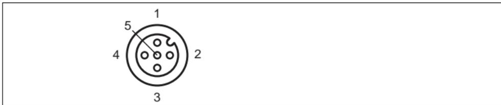
Figure 2.3: Trigger sensor connection layout
