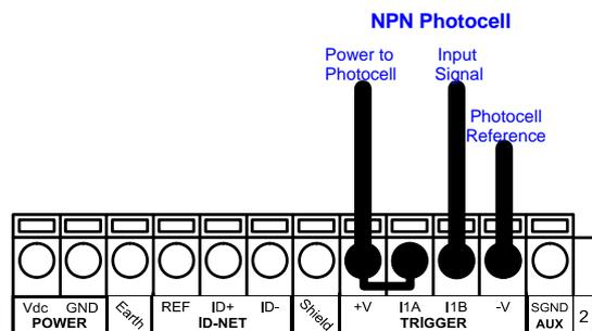
Figure 126 - NPN External Trigger Using CBX800 Power
