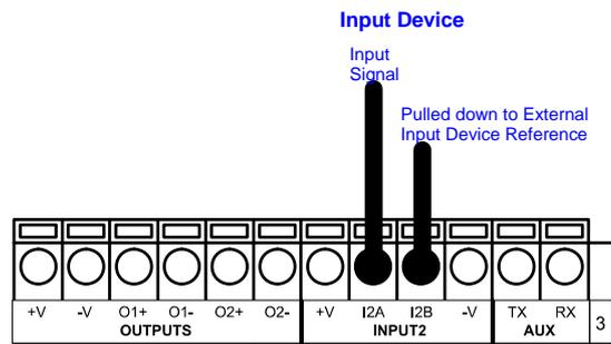
Figure 13 - PNP Input 2 Using External Power
