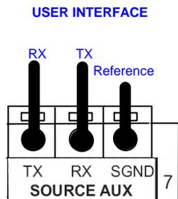
Figure 104 – Data Source Auxiliary Interface Connections
