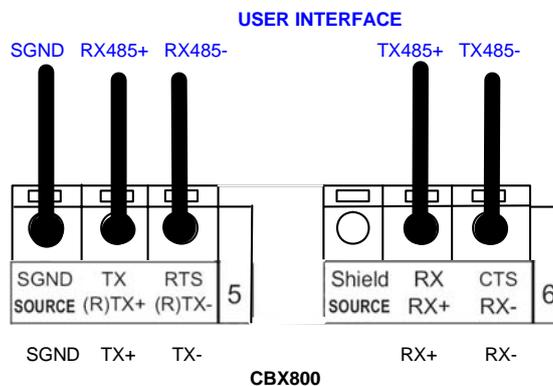
Figure 21 - RS485 Full-duplex Connections
