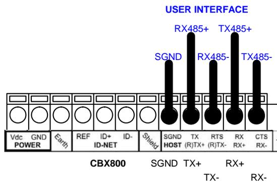
Figure 66 - RS485 Full-duplex Connections
