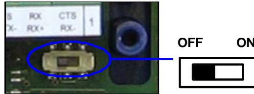
Figure 10 – RS485 HD Termination Resistance Switch
