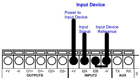
Figure 29 - PNP Input 2 Using CBX800 Power
