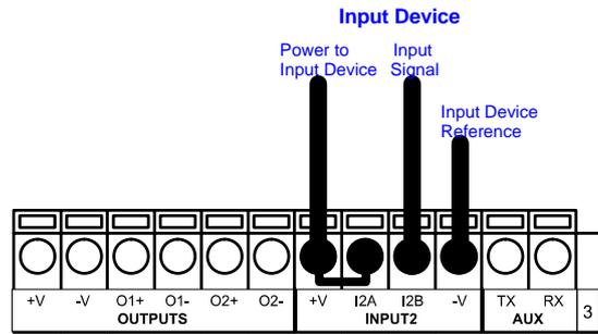
Figure 30 - NPN Input 2 Using CBX800 Power
