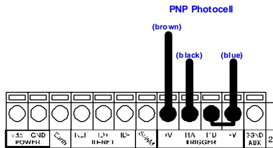
Figure 115 –External Trigger Using CBX800 Power
