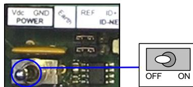
Figure 3 - Power Switch ON/OFF Positions
