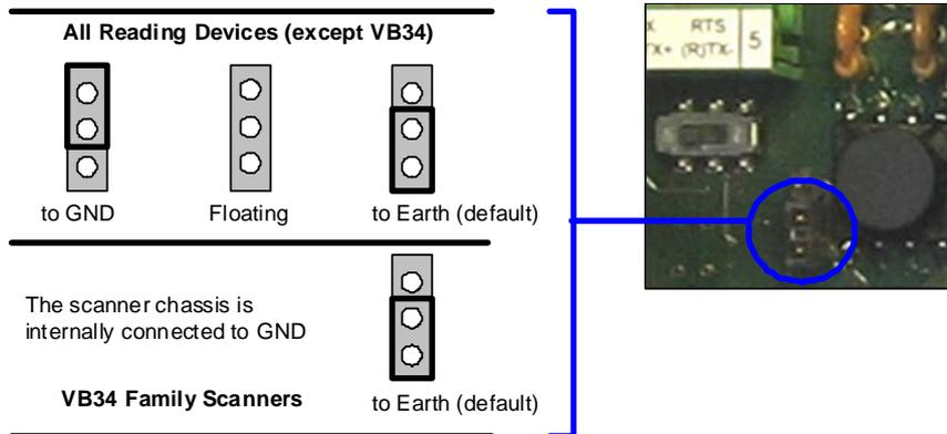
Figure 7 – Chassis Grounding
