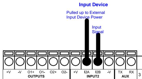
Figure 14 - NPN Input 2 Using External Power
