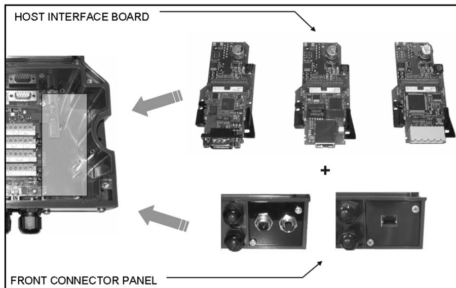
Figure 1 – CBX800 Front Connector Panel
