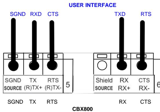
Figure 20 – RS232 Data Source Interface Connections
