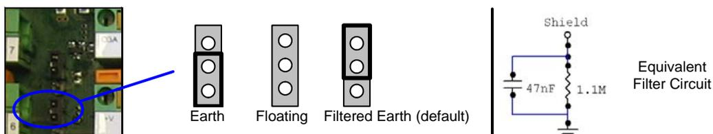
Figure 6– Source Shield Jumper Settings
