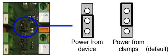
Figure 5–Power Source Jumper Settings
