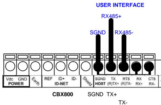
Figure 77 - RS485 Full-duplex Connections using Only TX Signals
