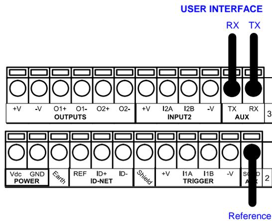
Figure 19 - RS232 Auxiliary Interface Connections
