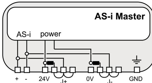
Figure 5.1: Terminals of a device with power supply 'N'
