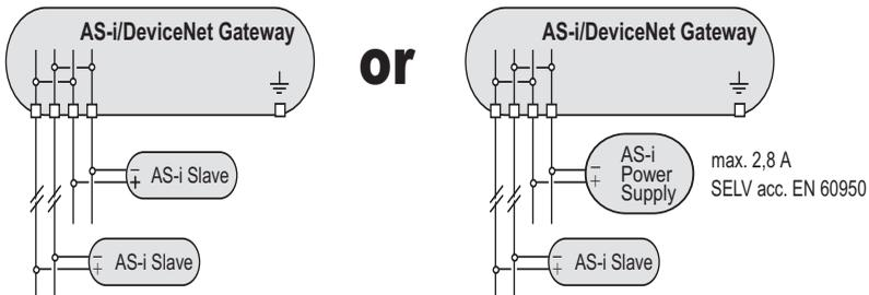
Figure 5.6: Terminals of a Device With Power Supply DeviceNet
