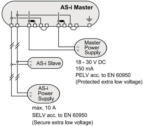
Figure 5.3: Operation with AS-i power supply
