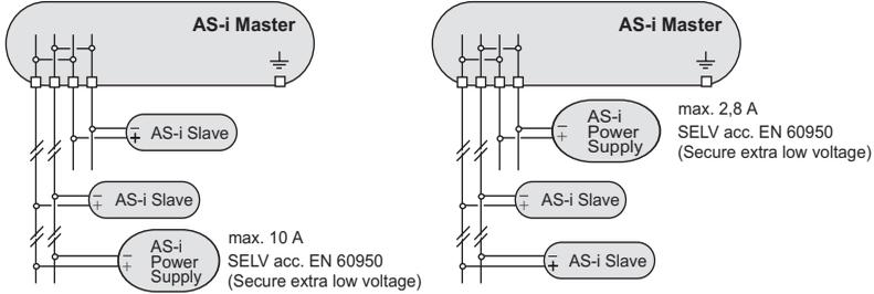
Figure 5.5: Connection samples for the AS-i power supply facilities
