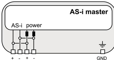
Figure 5.4: Terminals of a device with power supply 'A'
