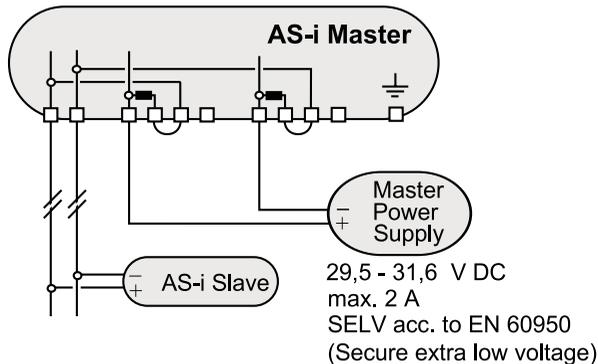
Figure 5.2: Operation without AS-i power supply
