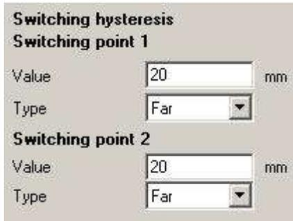
For each active switching point, a corresponding switching hysteresis in millimeter can be set. Make sure that the switching point with its corresponding switching hysteresis does not exceed the sensing range. Furthermore, there are four different types of switching hystereses:
