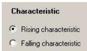
It is possible to set a rising or a falling characteristic. In the case of a rising characteristic, the current or the voltage at the analog output rises with increasing object distances. In the case of a falling characteristic, the current or voltage at the analog output falls with increasing object distances.
