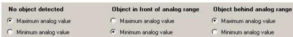
The behavior of the analog output outside the analog range can be set for the following three modes:
