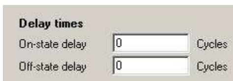
It is possible to delay switching on or off the output. Both delay times can be extended by an integer number of measuring cycles. The delay times can be set in the range from 0...255 measuring cycles.
