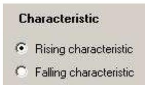
It is possible to set a rising or a falling characteristic. In the case of a rising characteristic, the current or the voltage at the analog output rises with increasing object distances. In the case of a falling characteristic, the current or voltage at the analog output falls with increasing object distances.
