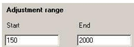
The adjustment range is the range where the selected range limit can be adjusted with the potentiometer. The start of the adjustment range corresponds to the selected range limit at left stop of the potentiometer. The end of the setting range corresponds to the selected range limit at right stop of the potentiometer. The adjustment range always refers to both potentiometers if they are active.
