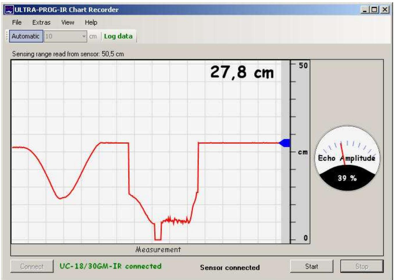
For measuring cycle times of more than 5 milliseconds, the data logger continuously records measured values without any loss of measuring cycles. The measured values are first filed in the RAM of the PC. After completion of the recording phase, the user can assign a file name and path for the filing on a storage medium. The recording format is CSV (Comma-Separated Values) and can be read and processed with, for example, Microsoft Excel.
