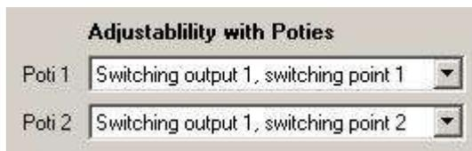
For potentiometer 1 and potentiometer 2, a range limit can be set that is adjustable with the respective potentiometer. It is also possible to deactivate one or both potentiometers.
