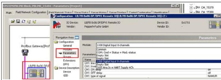
↳ The parameters of the selected remote I/O module are available for editing in the list below. Configure the parameters for each remote I/O module as required.
