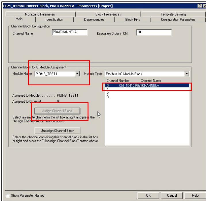
↳ The data of the remote I/O module is assigned to the controller and can be used for process control.
