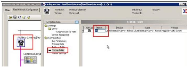
3. Click **Apply** to apply the new address to the PROFIBUS slave and click **OK** to close the window.
