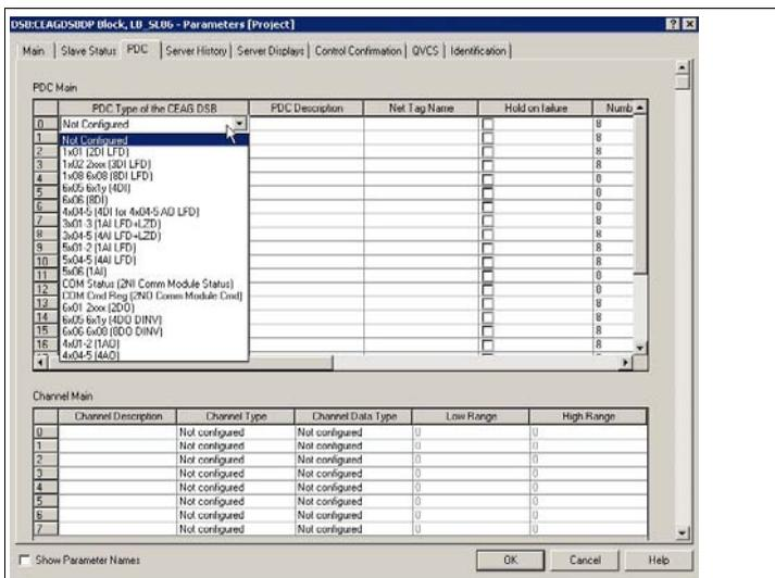
8. To avoid errors, enter the low range and high range for the global status register. Note that it is not used as an analog value.
