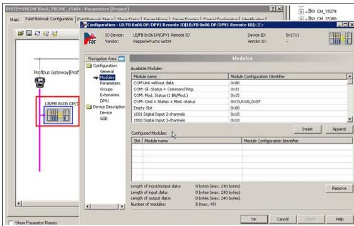
3. To configure a remote I/O module, select a module from the **Available Modules** list and click **Insert** to add the selected module to the **Configured Modules** list.
