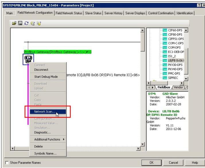
↳ The hardware that is currently connected to the PROFIBUS gateway is displayed.
