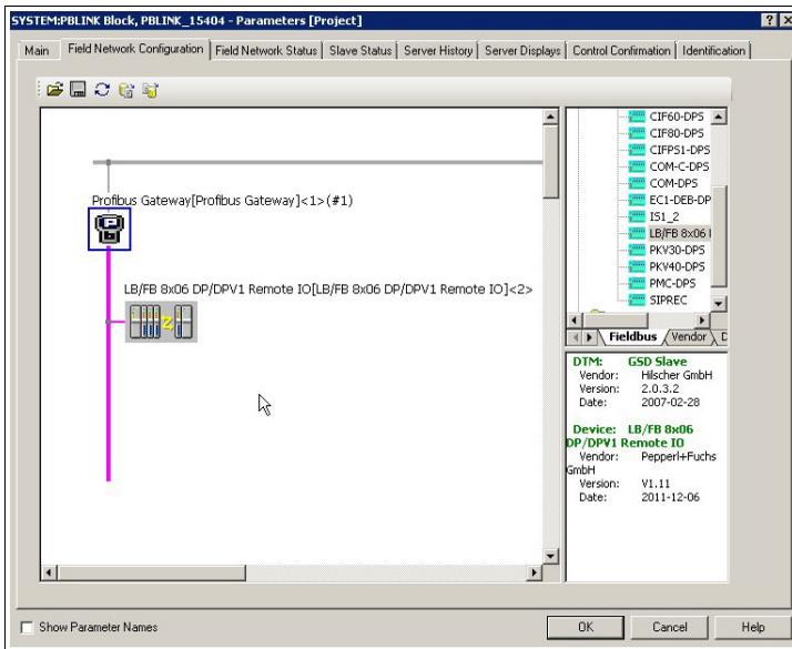
↳ The field unit is added to the PROFIBUS line and the address is defined automatically.
