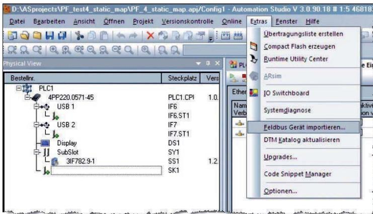
A new window will open. Go to the option "POWERLINK Geräte" and select the correct XDD file for the encoder used.
