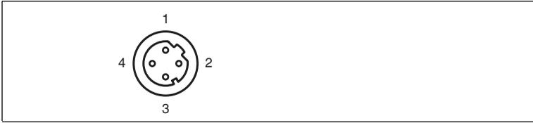
Figure 5.2 Ethernet connection layout
