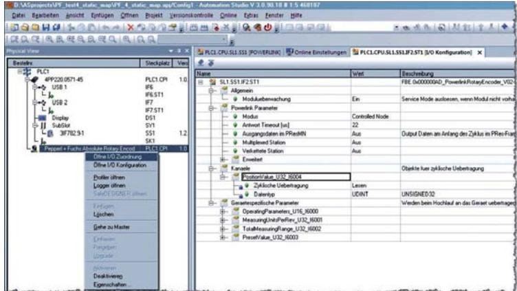
The transferred position value and the device status appear on the right-hand side of the open window.
