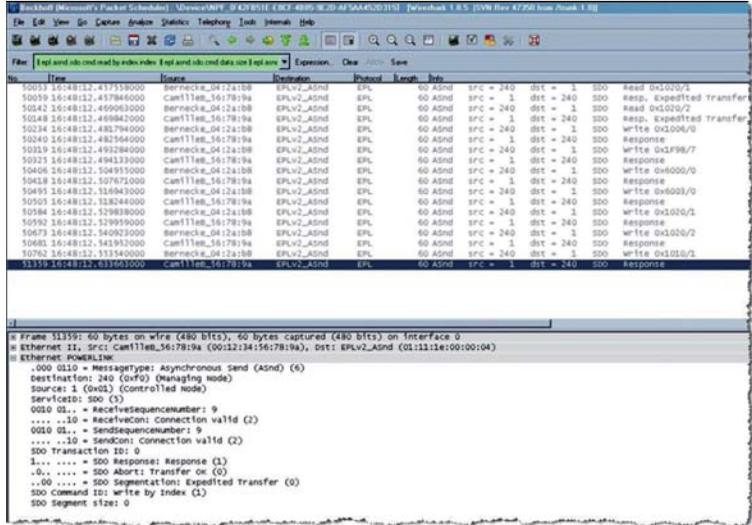
In this screenshot, you can see a log of configuration telegrams (SDO messages). The telegrams, as well as the associated object with subindex, are displayed in the right-hand column. This makes it easy to check which parameters/objects of the rotary encoder are set. To display this type of view, you must set the filter in the following way:
