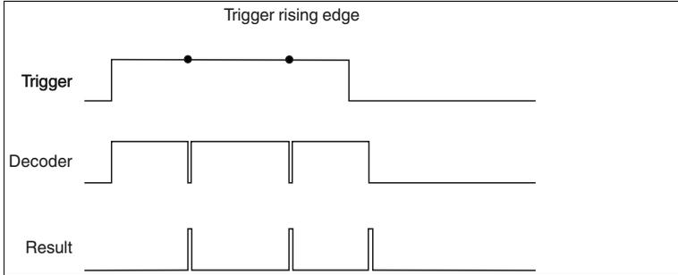
Figure 7.2 Pulse diagram trigger rising edge and level
