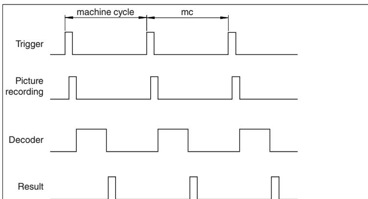
Figure 7.4 Pulse diagram single trigger
