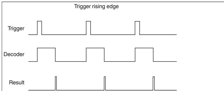
Figure 7.1 Pulse diagram trigger rising edge
