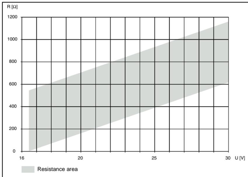
If a current output is operated as a source, the load resistance must be between  $0\ \Omega$  and  $550\ \Omega$ . Further information on connecting the UT2 can be found in the data sheet and in the operating instructions for the K-System on our Internet page [www.pepperl-fuchs.com/pa](http://www.pepperl-fuchs.com/pa) (under product search, enter \*UT2\*).
