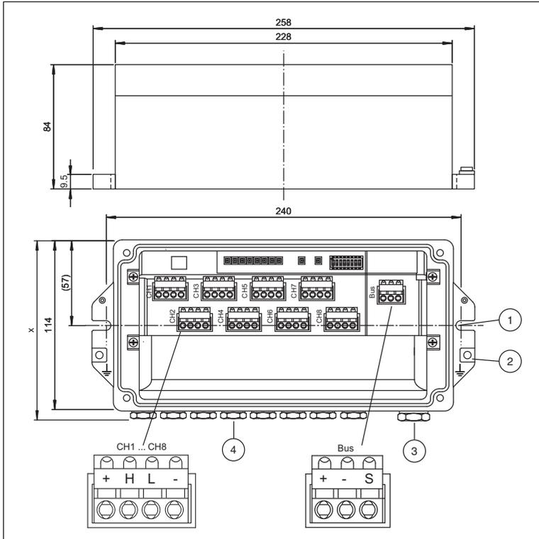
1. Notch for fixing the Temperature Multi-Input Device housing with M6 screw
