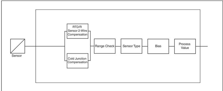
Figure 4.9 Signal measurement dataflow
