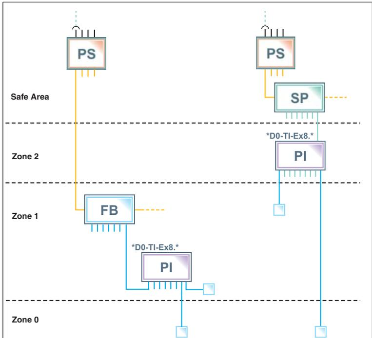
Figure 2.1 Installation options for the Temperature Multi-Input Device in the hazardous area
