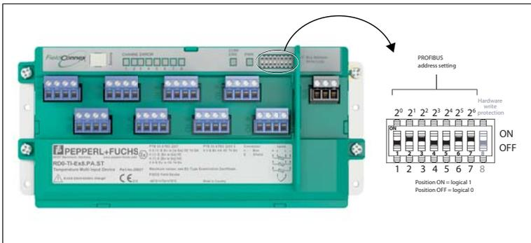
Figure 3.7 DIP switches to set the PROFIBUS address on the device
