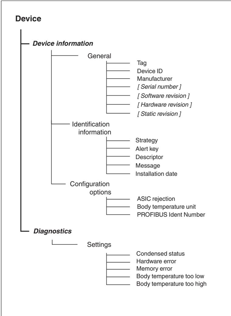
Figure 3.11 DTM menu structure: Device-specific
