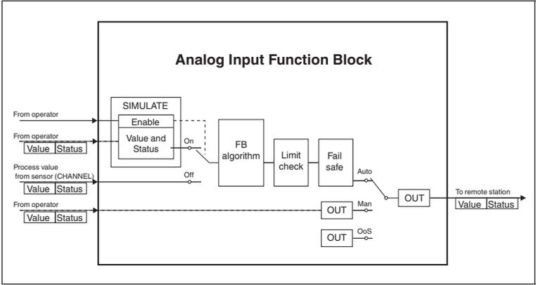
Figure 4.10 Analog input function block
