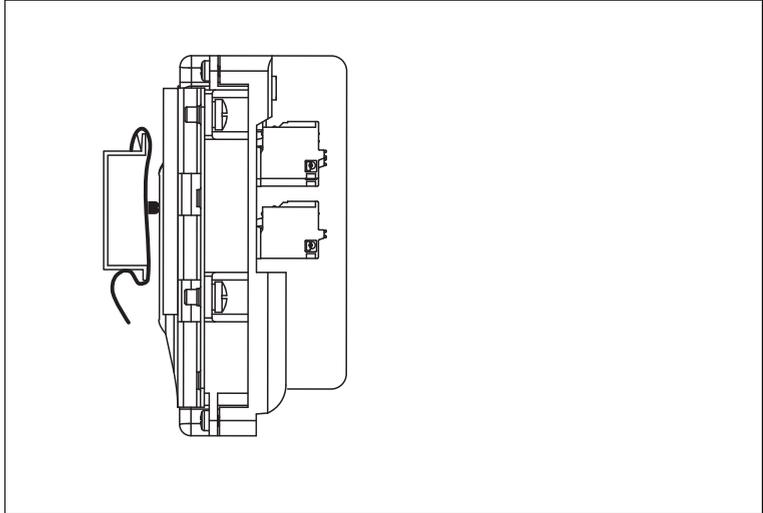
Ensure that the device is firmly fixed on the DIN rail.
