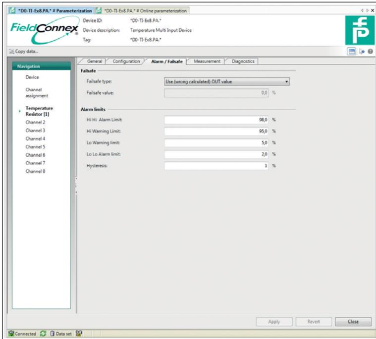
Figure 4.13 Tab alarm/failsafe
