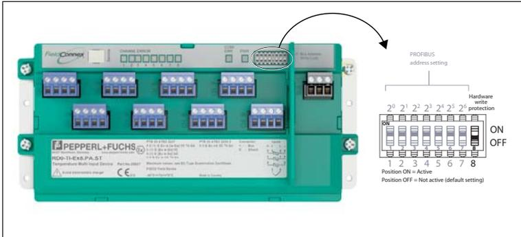
Figure 3.6 Dip switch 8 to activate the hardware write protection
