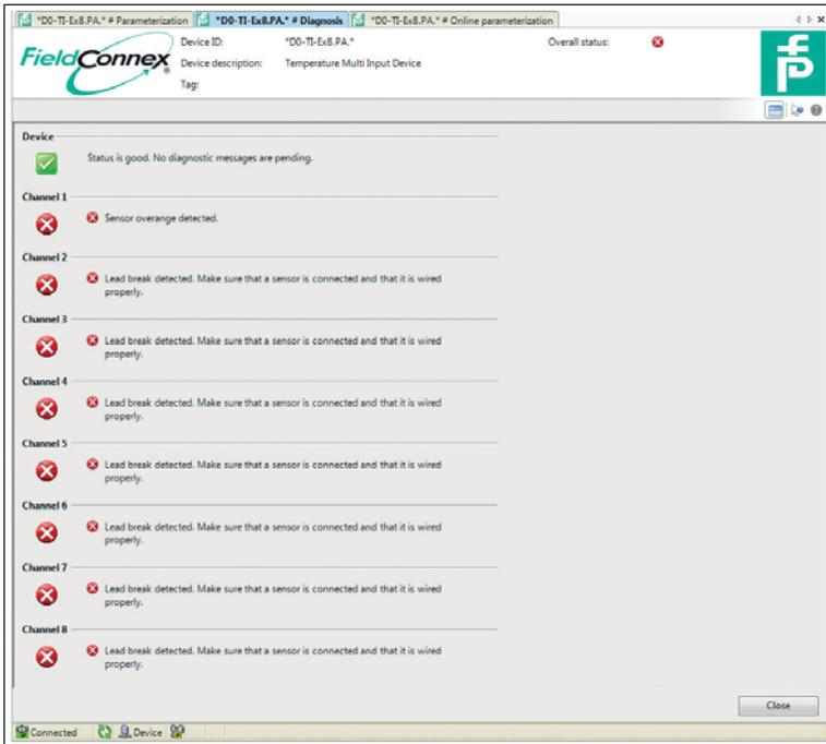
The DTM dialog diagnosis enables you to identify errors as efficiently as possible. Diagnosis displays the NAMUR icon for the device and each channel, as well as a list of active faults. The condensed status of the device can be configured via **Device > Diagnostics**. For more information, see chapter 4.1.2 and see chapter 4.2.5.
