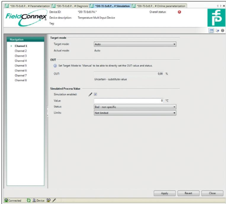
Figure 4.16 Tab simulation with target mode set to auto.
