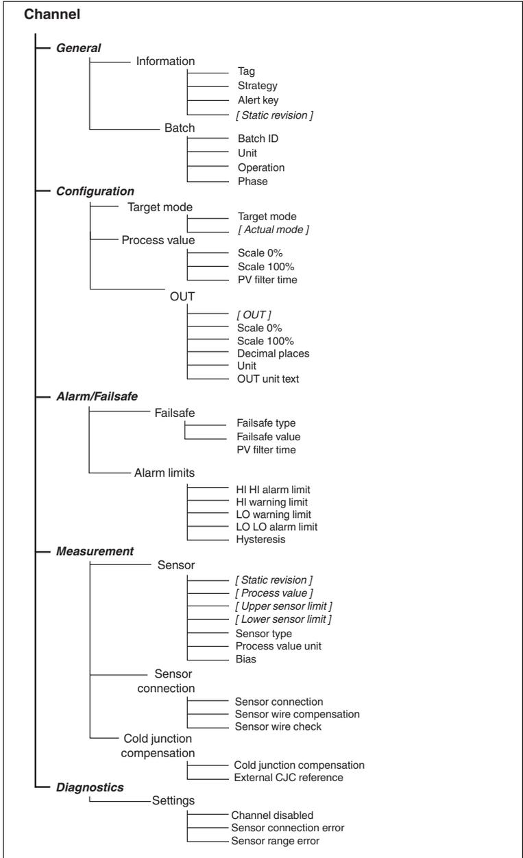
Figure 3.12 DTM menu structure: Channel-specific
