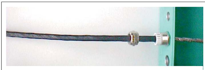
3. Remove the inner plastic piece and slip it onto the cable: move it far enough over the cable, so it completely surrounds the cable insulation. Ensure that no cable insulation protrudes behind the inner plastic piece.
