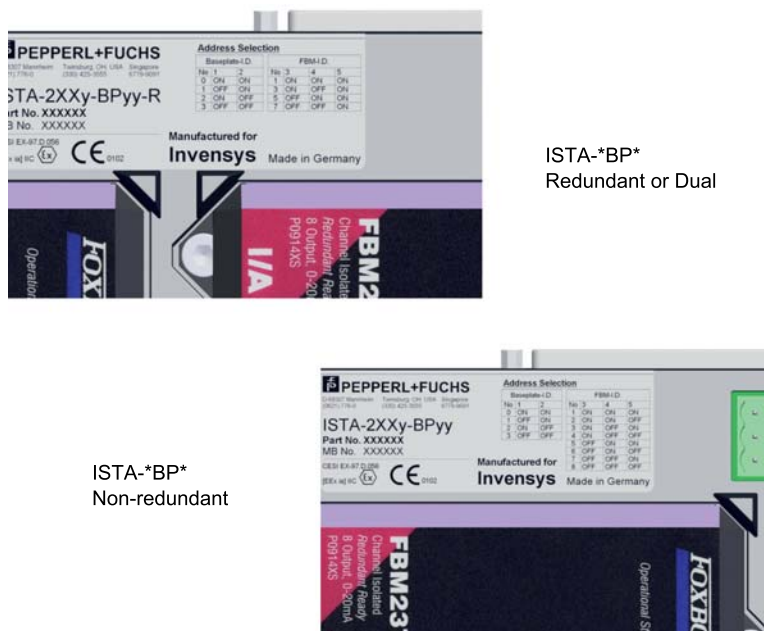
Figure 3-15. Addressing a Non-Redundant, Dual or Redundant ISTA-*BP*
