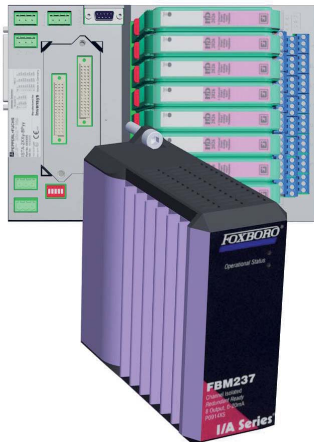
Figure 3-3. Mounting of FBM on ISTA-*BP*
