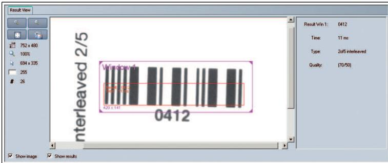
Figure 7.23 Result View screen with image display and result display
