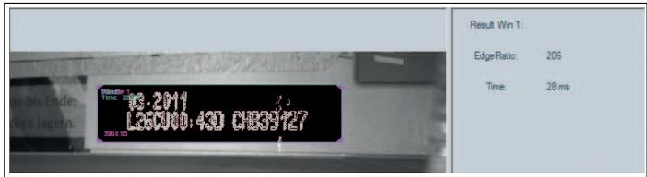
↳ The resulting image is shown in the image display. Edge transitions are displayed in graphic form in the resulting image. The resulting value is shown in the image display under **Result Win 1**.
