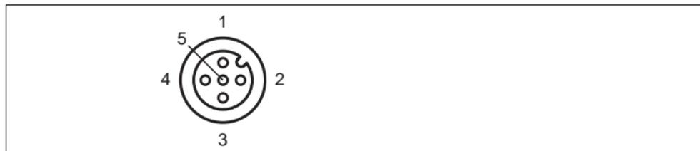
Figure 2.8 Connection layout RS 232
