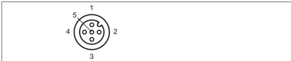
Figure 2.4 RS 232 interface connection layout
