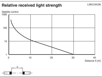
The thru-beam sensor requires a pair of devices for operation, comprising a light transmitter and a light receiver. The emitter and receiver must be arranged in optical alignment with each other. The infrared light from the emitter is detected by the receiver and evaluated.
