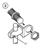
Tighten the screw fully after the sensor has been mounted and aligned.
