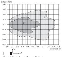
Curve 1: flat surface 100 mm x 100 mm Curve 2: round bar,  $\varnothing$  25 mm
