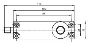
Bore hole and countersinking for screws/hexagon M4
