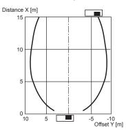
Permissible distance (offset) between the optical axis of the emitter and receiver.
