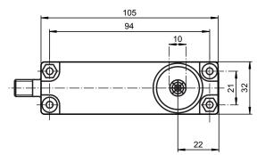
Bore hole and countersinking for screws/hexagon M4
