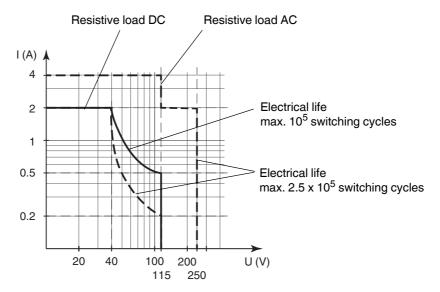
The maximum number of switching cycles is depending on the electrical load and may be higher when reduced currents and voltages are applied.
